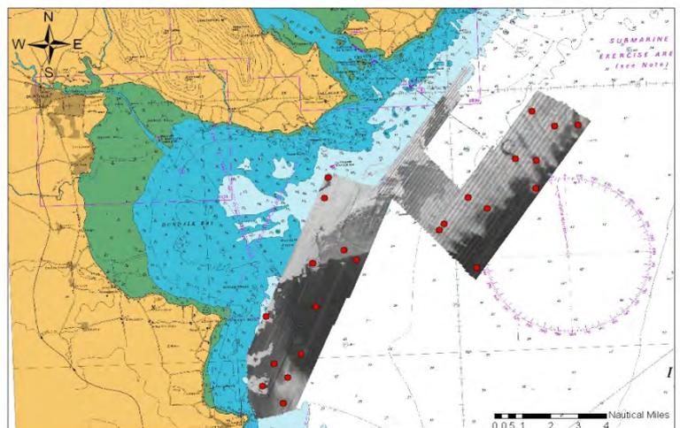
Figure 2: Geo-coded backscatter data acquired during survey operations onboard the *Celtic Voyager* between 2nd and 13th September 2011. This data will enable seabed classification and the identification of sediment types. The red dots show the sites where the team collected samples for ground truthing.
