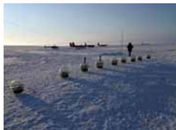
Clear-hulled GPS buoys being prepared at Alert station in northern Ellesmere Island. The buoys all report their position via satellite in support of studies of the movement of sea ice in the Arctic Ocean and the adjacent Nares Strait. Two buoys also report barometric pressure for use by the global weather forecasting community.
