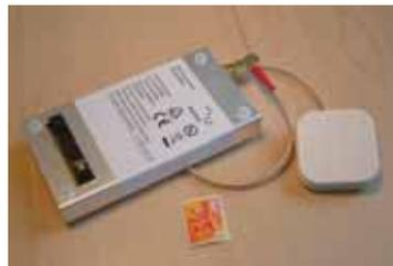
An Iridium 9601 satellite modem and antenna. This device is transforming our ability to interact with and receive data from remote instruments anywhere in the world.
